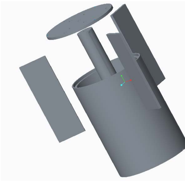
Figure 4: Exploded view of experimental enclosure displaying fins, core, top cap and enclosure.
